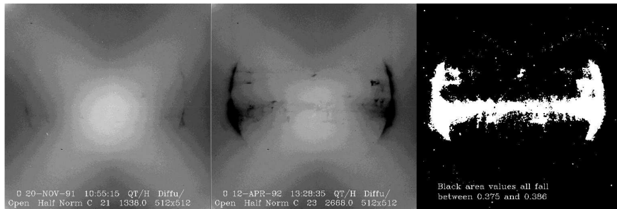
Figure 24. SXT diffuser images. Increased radiation-damaged area is evident in the center (later) image. In the rightmost panel the black portion shows the area of the CCD in which the signal decrease is very uniform, falling between 61.4 and 62.5 percent.
