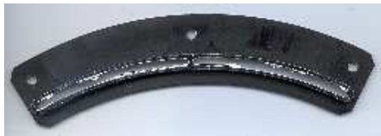
Figure 15. SXT entrance filter frame. The filter membrane itself has been destroyed in testing, showing the catastrophic degradation typical of the failure of thin films of this type.
