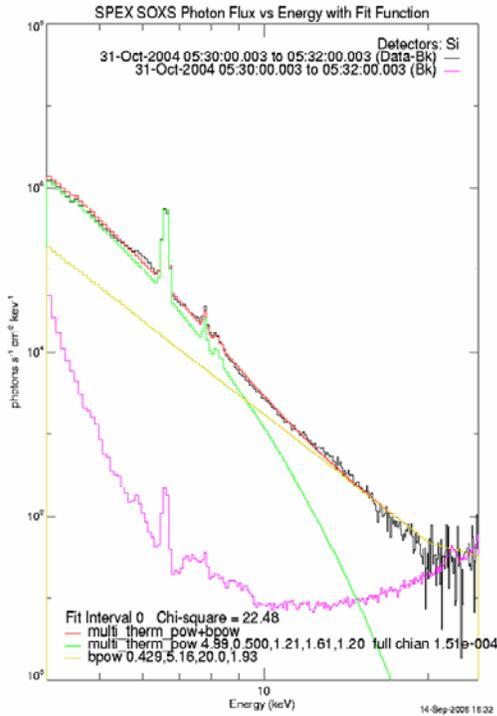
**Fig. 4.** The X-ray photon spectra of 31 October 2004 at 05:30:59 UT in 4 – 25 keV. The spectrum is fitted with multi-thermal power law plus non-thermal break power law. Differential emission measure, temperature of the plasma and the photon index are measured from the fit. X-axis error bar is channel width of 0.082 keV.
