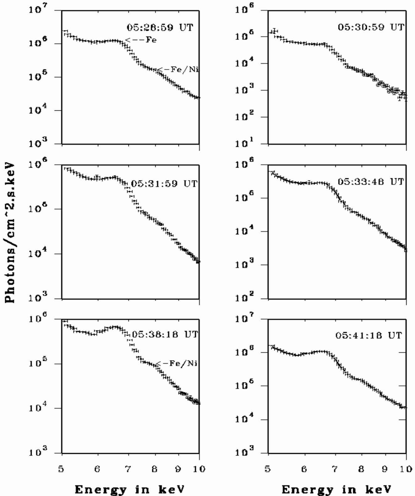
**Fig. 3.** Sequence of X-ray photon spectrum in the energy range 5 – 10 keV of 31 October 2004 flare showing evolution of Fe and Fe/Ni line features. X-axis error bar is channel width of 0.082 keV, while Y-axis error bar is  $\pm 1\sigma$  of the photon flux in the given channel.
