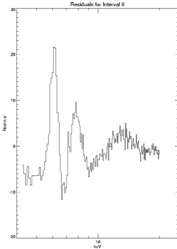
**Fig. 5.** The residual (difference) counts of multi-thermal power law plus non-thermal break power law fit (cf. Fig. 4).
