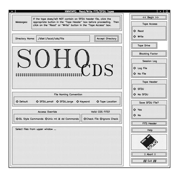
Figure 1: The XWINTAPE widget as it appears at the start of an archiving run.
