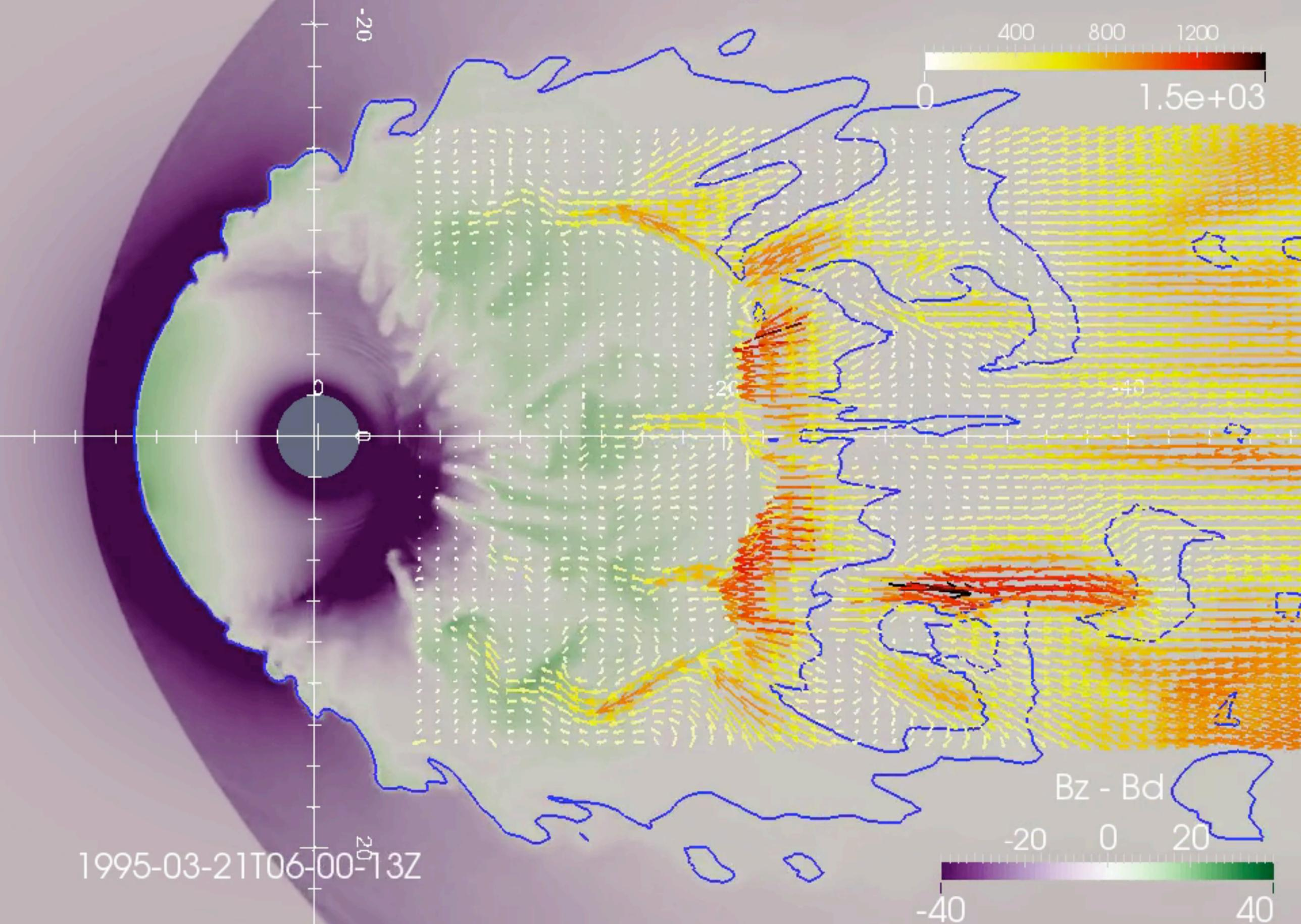
This high resolution magnetosphere simulation by Mike Wiltberger shows the structure of the BBFs in the magnetotail. The purple/green color table shows the difference between the dipolar magnetic field and the magnetic field in the simulation. The red/yellow color table shows the speeds of the bursty bulk flows. The morphology is remarkably similar to the SADs in the corona.
